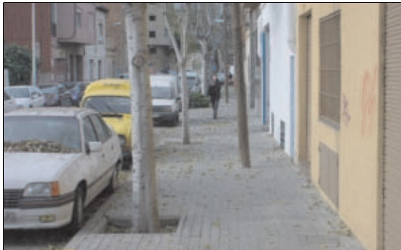
Picture 013 > Elements which are not aligned with and placed on the edge of the pavement can be the cause of an accident or disorientation of visually-impaired people
