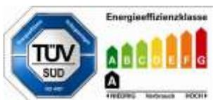
Previously only seen on household appliances: The new energy-efficiency label for lift systems as per VDI Guideline 4707 indicates the energy-efficiency class.
